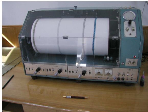
Figure 2: (a) A general circuit diagram for the observation equipment; (b) A photograph of the electrodes and the DJ-1 recorder. The body of the sensor of the electrodes is made of high quality Cr18Ni9C stainless steel. The water-proof pipe (white) will cover the whole screened transmission cables (black) when the electrodes are installed; (c) The DJ-1 recorder.
